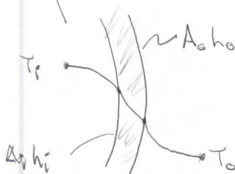
$$R_i = \frac{1}{h_i A_i} \quad R_{wall} \quad R_o = \frac{1}{h_o A_o}$$
